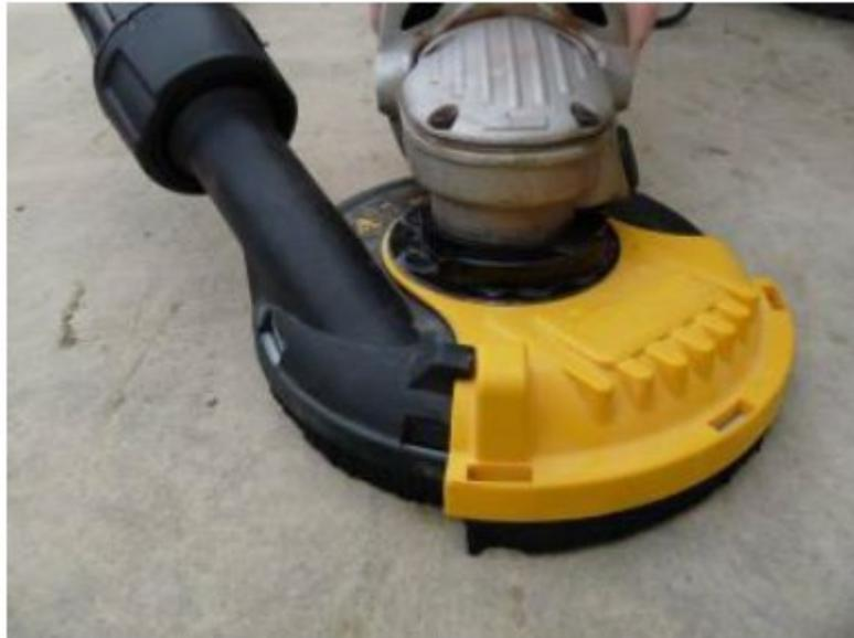
*Grinder with on tool extraction – UK HSE*
