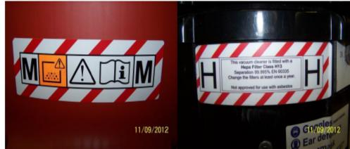
Figure 4 Label on M and H class extraction units (Source HSE, GB)
