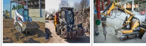
Good Practice – Utility vehicle cabin fitted with in-cab ventilation and material wetted before loading and transportation (MTS group Ltd, GB and JCB, GB)
