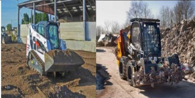
**Good Practice** – Utility vehicle cabin fitted with in-cab ventilation and material wetted before loading and transportation (MTS group Ltd, GB and JCB, GB)
