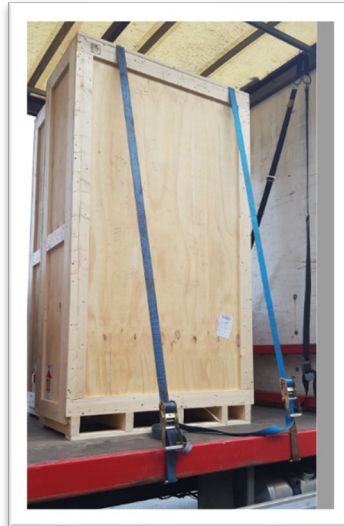
Figure 3 – Example of Strapping on a Curtain Side Trailer
