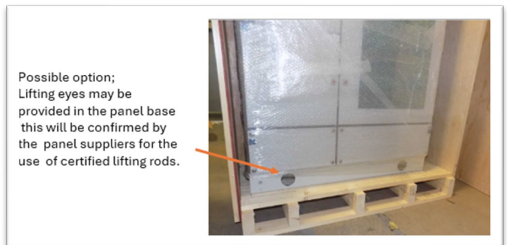
Figure 12 - Access Points for Lifting (with removable covers)
