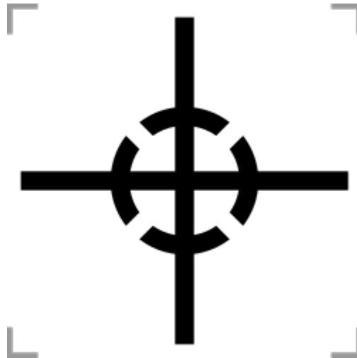
Figure 7 - Example of Centre of Gravity Indicator to ISO 7000-0627
