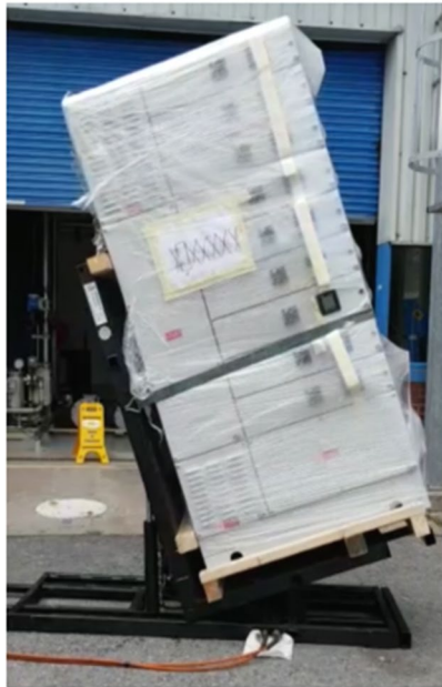
Image of Panel Tilter transferring to its horizontal position while laden with Panel Cubicle.
