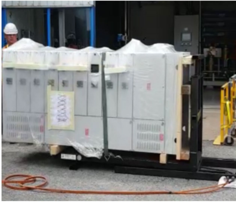
Image of Panel Tilter in the horizontal position laden with Panel Cubicle.
