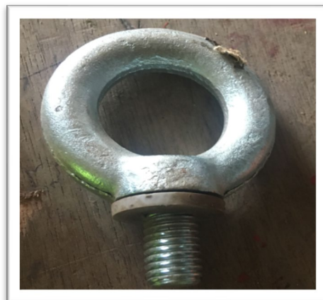
Figure 13 - Example of a Lifting Lug
