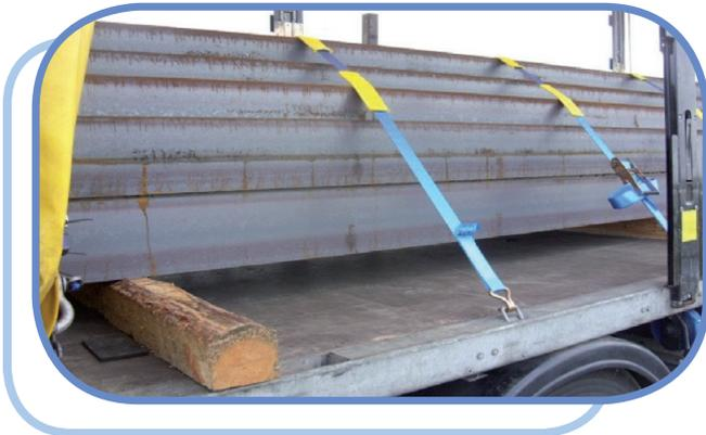
Figure 8. Correct use of edge protectors on web lashings
