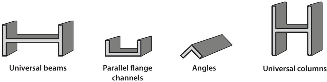
Figure 1. Examples of structural steel sections
