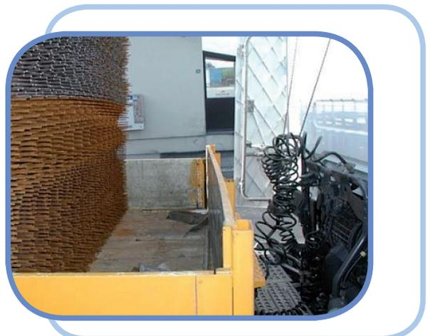
Figure 5. Inadequate headboard: No Blocking capacity
