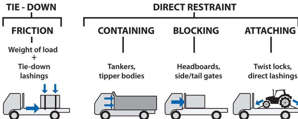
Figure 2. Load restraint methods (To control forward motion)
