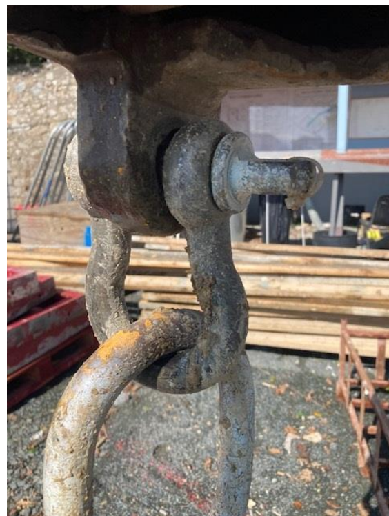
Shackle fully tightened on Excavator
