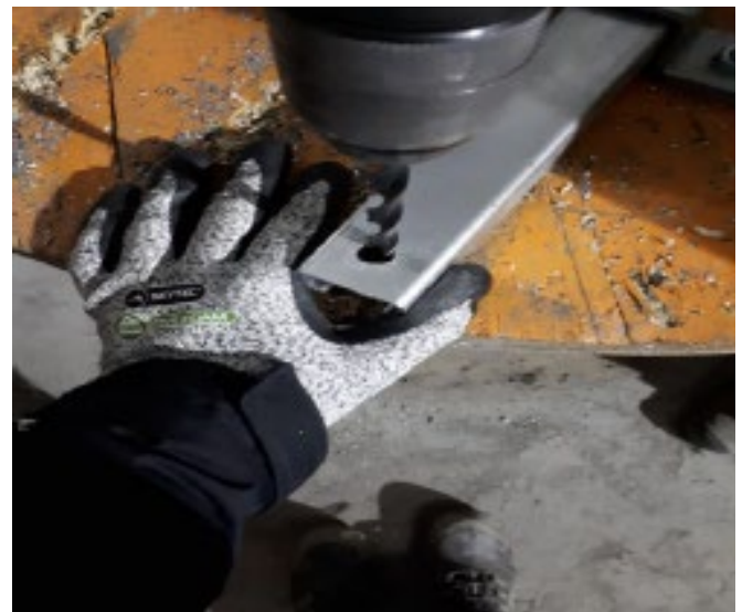
Figure 2: Reconstruction of hand placement, which resulted in injury
