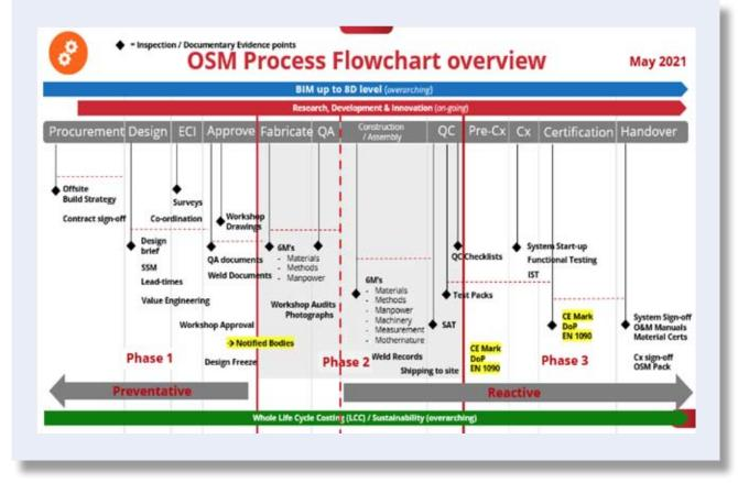
Figure 8: Offsite Manufacturing (OSM) Process flow diagram<sup>®</sup> Courtesy of Kyron Innovative Technologies Limited – May 2021 (Copyrighted – though reproduced with kind permission)
