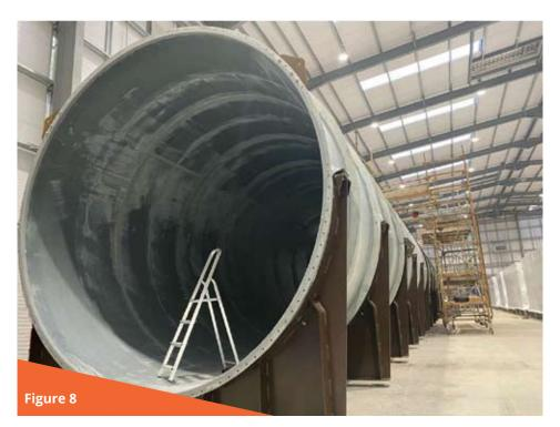
Breffni Ductwork fabrication offsite for a Semiconductor facility 8th March 2021
